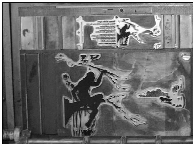
The black plates in position on the press. The dust jacket and bookmark were printed at the same time.
