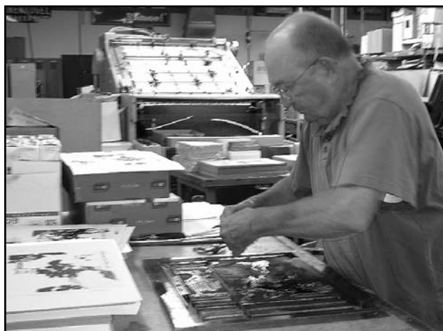
John sets up the plates in the chase, the frame which holds them in place on the press.
